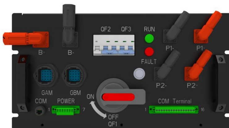
High-voltage Box Panel Layout
